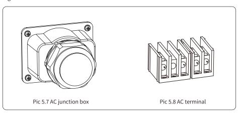
2) Connect the cable through the junction box, waterproof jacket, and insert into the terminal (The picture Pic 5.9 shows the connection mode of three phase lines connected to the junction box, ground wire screwed on the inverter shell), and use hexagon screwdriver to presses the wiring harness to the connect terminal as shown in Pic 5.10.
