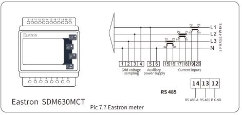
Inverter Solar Panel array AC Breaker RS 485 Male connector <u>4</u> <sub>485\_B</sub> vcc\_5v \_1 Home load RS 485 Female connector <u>3</u> 485\_A GND -00000000 485 A 485 B meter RS485 Communication GND Generator Pic 7.8 Connection diagram of Eastron meter
